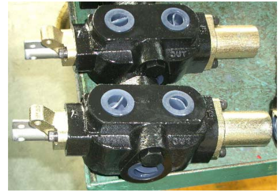
Log Splitter Valves
